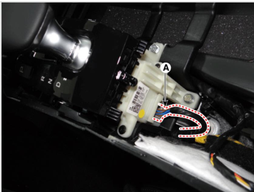
3. Loosen the E-shifter mounting screws (A).
