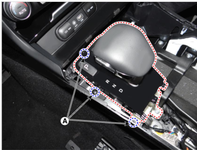
4. Loosen the E-shifter mounting bolts (A).
